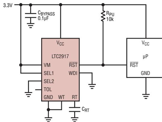
**Figure 11. A 3.3V, -10% tolerance supply monitor with disabled watchdog**
