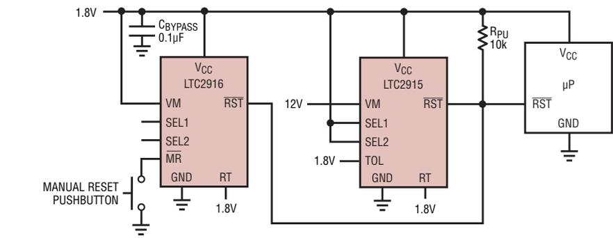
**Figure 7. Dual supply monitor (1.8V and 12V) with manual reset and 200ms Reset timeout**
