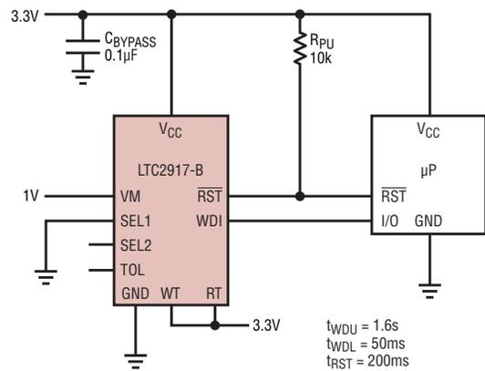
**Figure 9. A 1V supply monitor with windowed watchdog timeout and internal timers selected**
