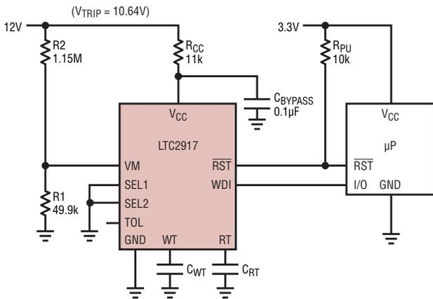
**Figure 8. A 12V supply monitor powered from 12V, utilizing the internal shunt regulator with 3.3V logic out**
