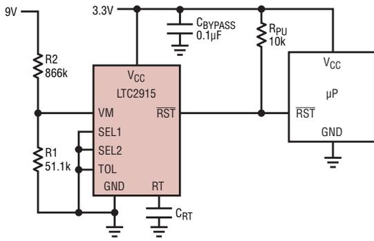
Figure 3. A 9V, -15% tolerance supply monitor with 3.3V logic out
