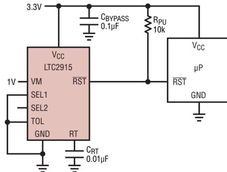
Figure 4. A 1V, -15% tolerance supply monitor with 90ms timeout
