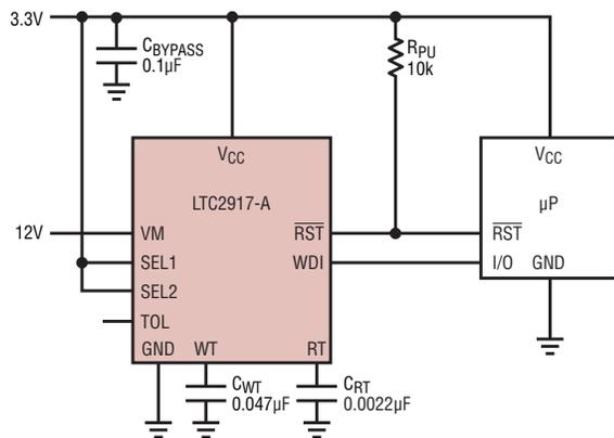
**Figure 10. A 12V supply monitor with 20ms reset timeout and 3.4s watchdog timeout, with 3.3V logic out**
