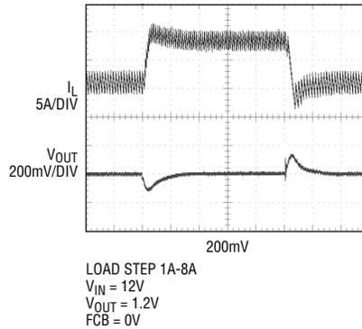
**Figure 3. Transient response for the typical LTC3608 application represented in Figure 1 with a load step of 1A to 8A**
