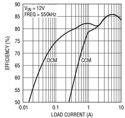
**Figure 2. Efficiencies for a typical LTC3608 application in discontinuous conduction mode (DCM) and continuous conduction mode (CCM)**
