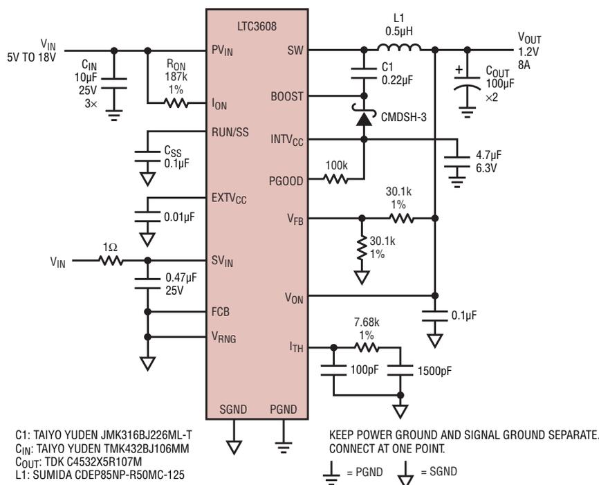
Figure 1. Typical application of the LTC3608
