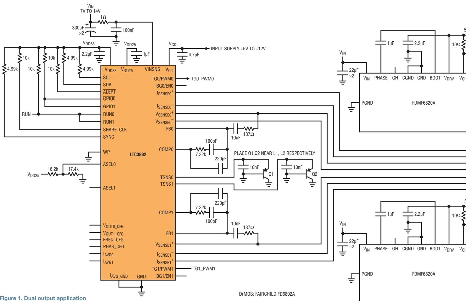
Figure 1. Dual output application using DrMOS to develop over 90W of output power
