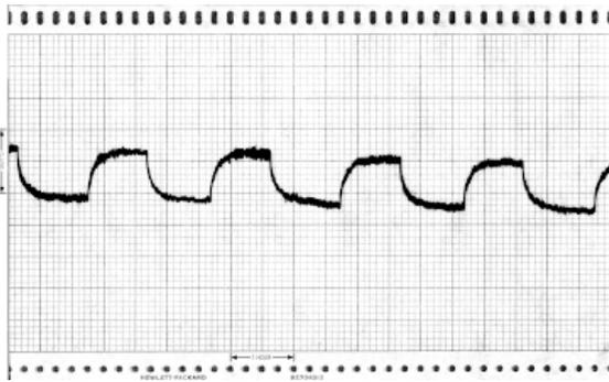
**Figure 10.** Long-term cooling mode stability measured in environment that steps 20 degrees above ambient every hour. Data shows resulting 0.008°C peak-to-peak variation, indicating thermal gain of 2500. The 0.0025°C baseline tilt over plot length derives from varying ambient temperature.
