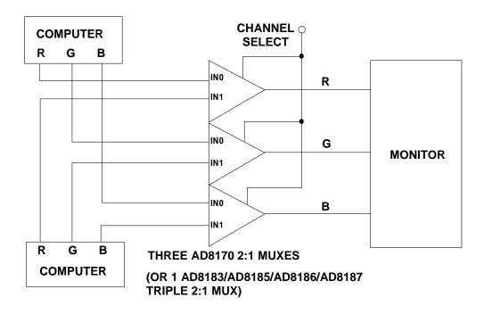
Figure 3: Dual Source RGB Multiplexer Using Three 2:1 Muxes
