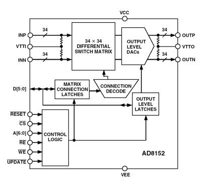
Figure 6: AD8152 3.2-Gbps Asynchronous Digital Crosspoint Switch
