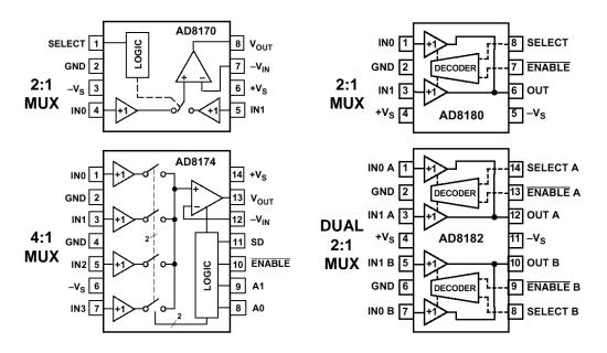
Figure 1: AD8170/8174/8180/8182 Bipolar Video Multiplexers
