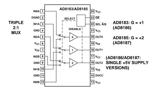
Figure 2: AD8183/AD8185 Triple 2:1 Video Multiplexers
