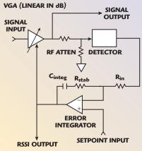
age. This is applied to the control input of the VGA. The attenuator shown between the VGA and the detector is used to align the maxi-
