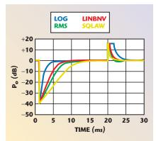
▲ Fig. 2 Simulated response of AGC loop to large amplitude steps for various detectors.
