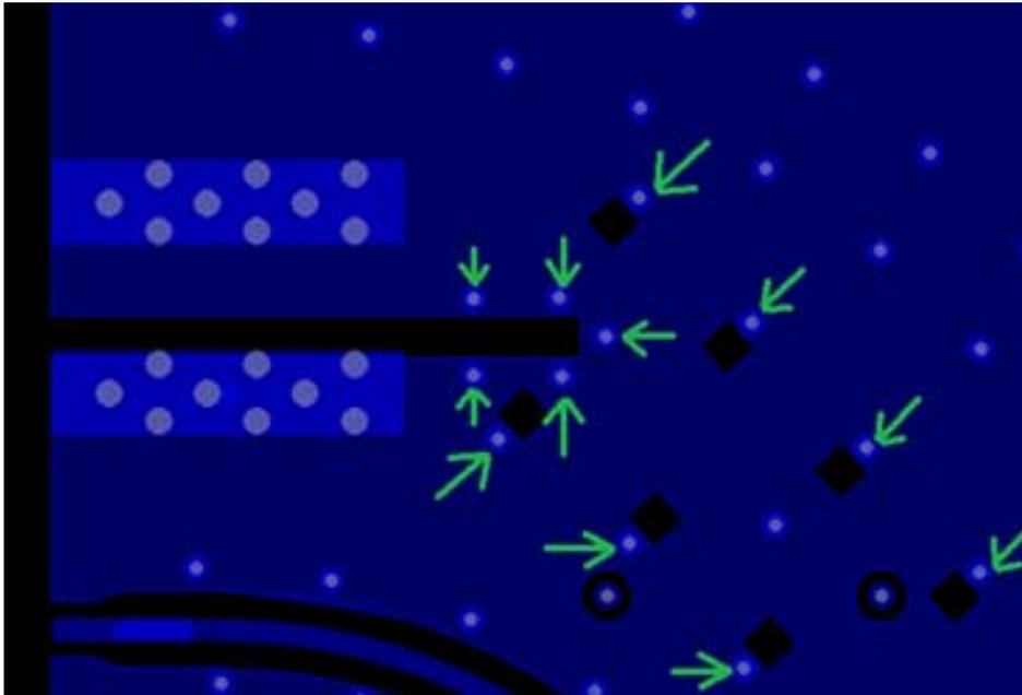
Figure 171. Current Steering Vias Placed Near Isolation Slots and Apertures
