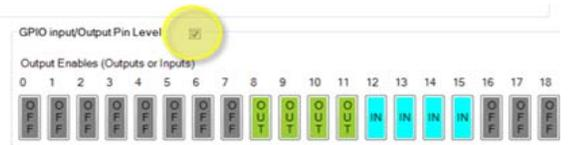
Figure 196. Selecting GPIO Pin Status: Output, Input, or Disabled
