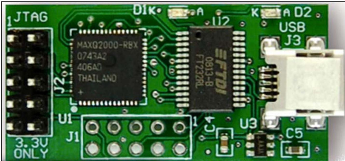
Figure 3. The Maxim USB-JTAG adapter (MAXQUSBTAG-KIT).
