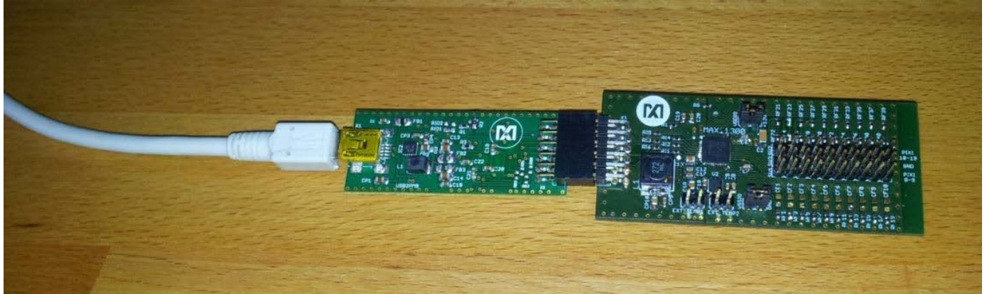
Figure 16. MAX11300PMB1/Munich Connected to PC Through a USB Cable
