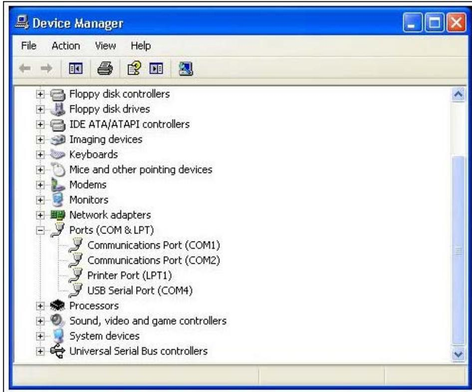
Figure 3. USB serial-port COM location in device manager.
