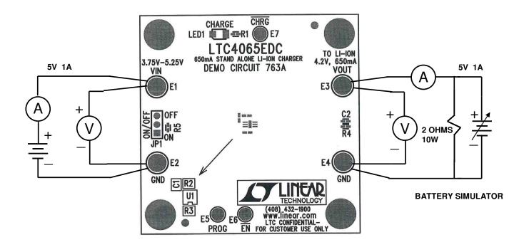
Figure 1. Proper Measurement Equipment Setup
