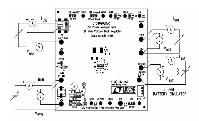
Figure 1. Proper Measurement Equipment Setup
