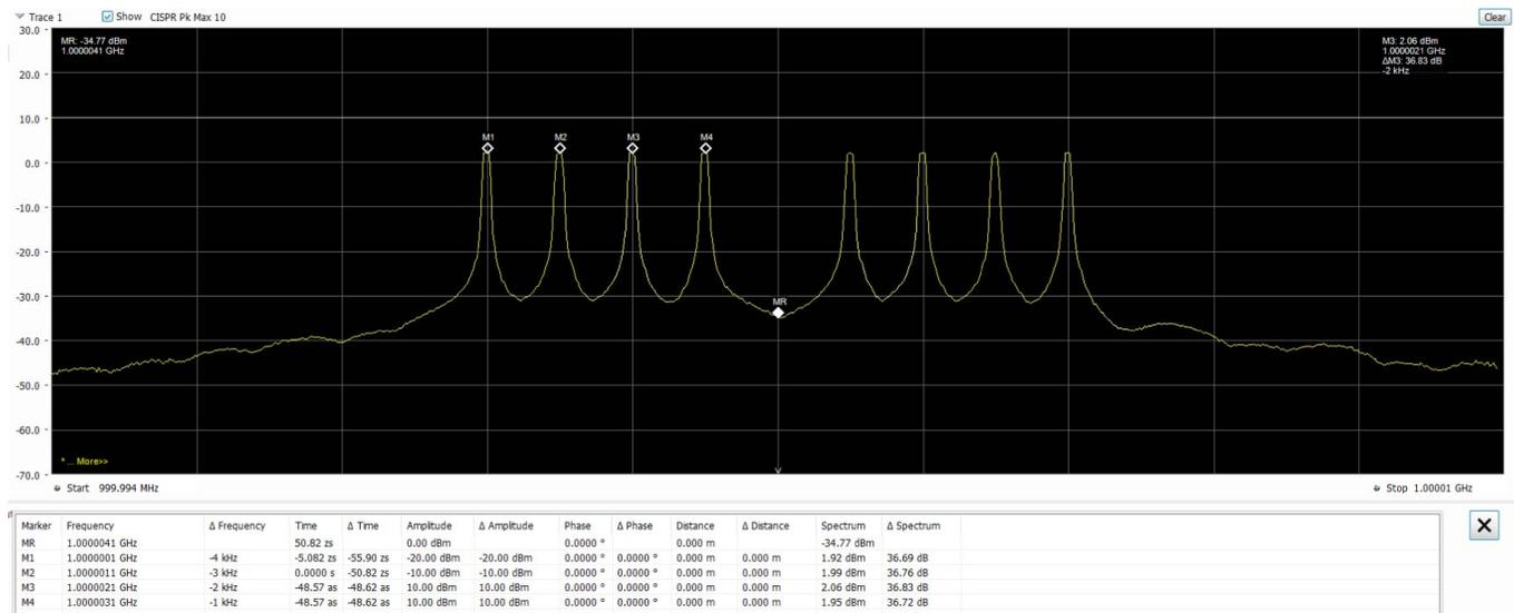
Figure 372. Transmitter TDD DMR with Frequency Hopping
