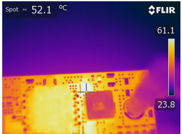
Figure 30. Thermal Image of SR1 at 48 V DC Input, 6 A Load, No Airflow, 1 Hour Soaking Time
