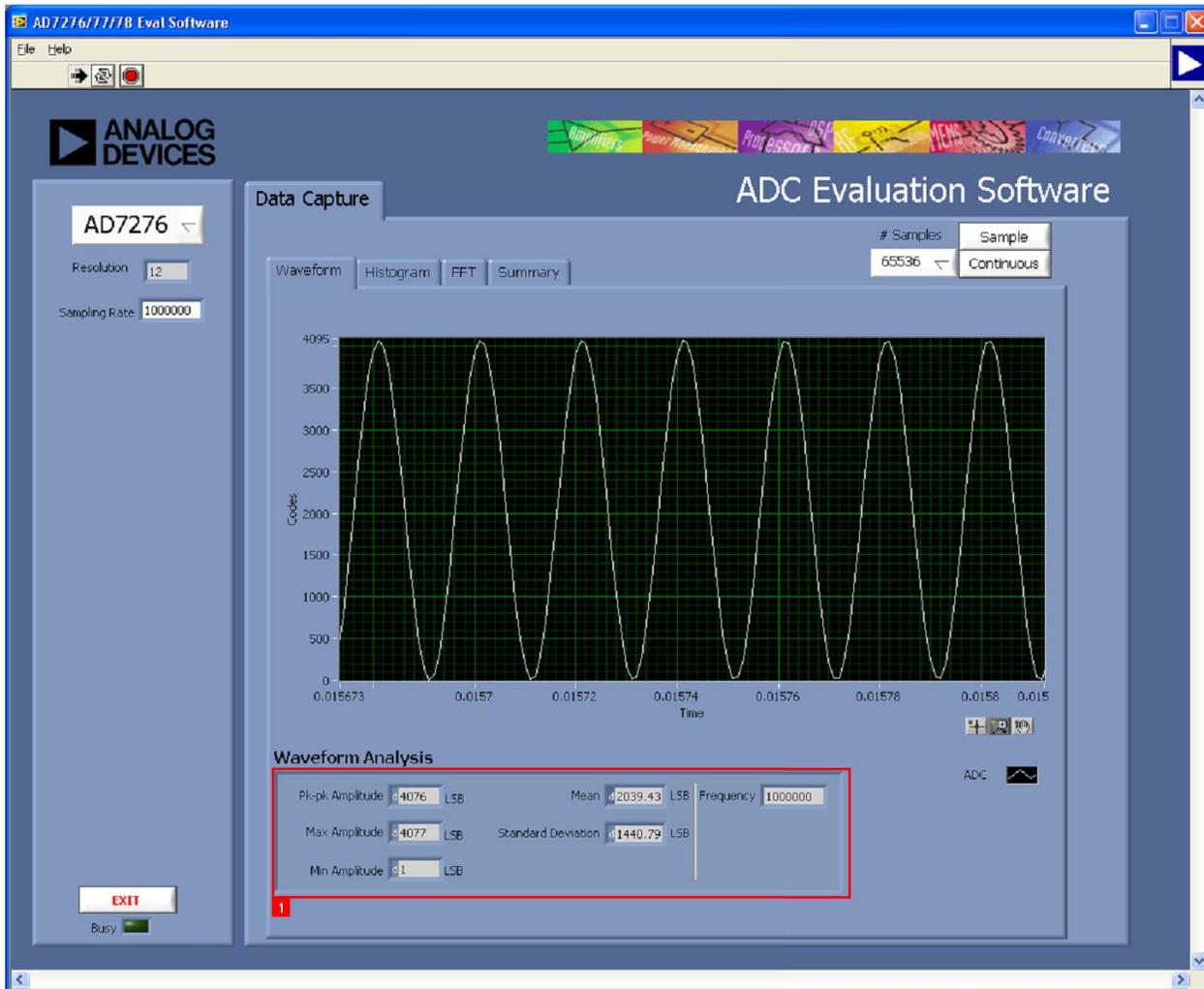
Figure 18. Waveform Tab
