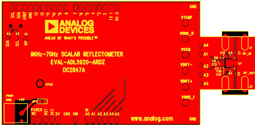
Figure 5. Layer 1 of the EVAL-ADL5920-ARDZ (DC2847A)
