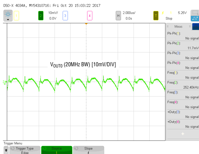
Figure 9. Output Voltage Ripple at V_{IN} = 12V , V_{OUT0} = 1.0V , I_{OUT0} = 10A
