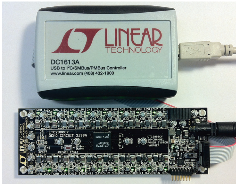
Figure 2. Connecting DC2198A Board and the DC1613 I 2 C/SMBus/PMBus Controller
