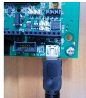
Figure 22. USB to UART Connection
