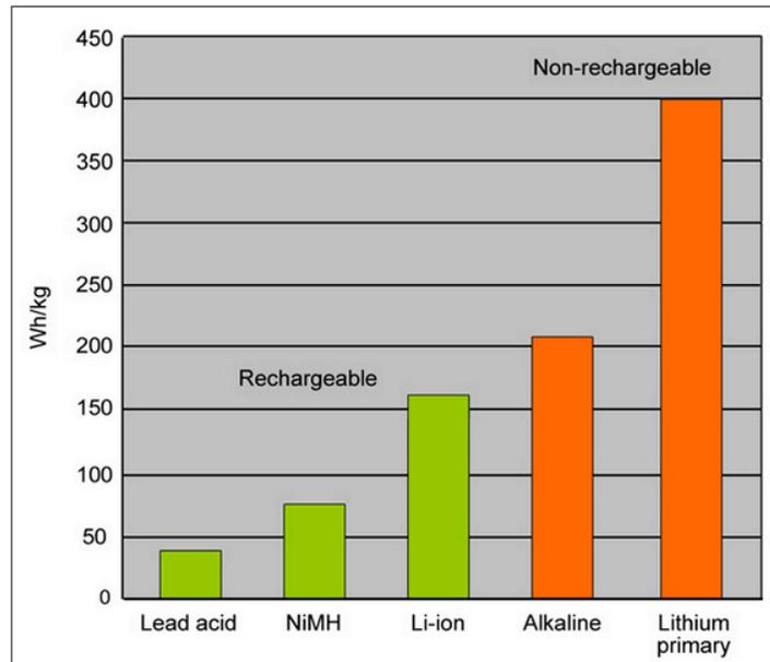
Figure 1. Energy Density of Rechargeable vs. Primary Cell Batteries
