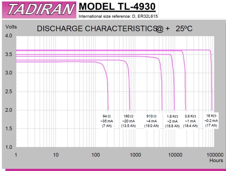
Figure 2. Discharge Curve for Tadiran Model TL-4930 Primary Cell
