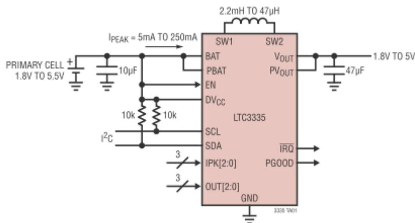
Figure 4. Simplified LTC3335 Application Schematic
