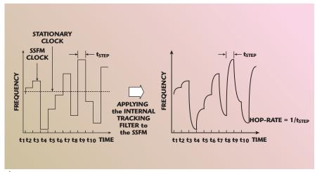
Fig. 2 Pseudorandom modulation and internal tracking filter of LTC6909.
