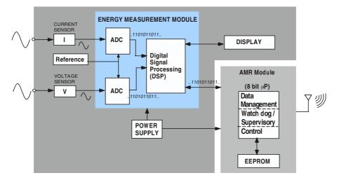
Figure 1: Functional block diagram of an electronic energy meter
