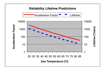
Figure 3. Acceleration factor and lifetime predictions in relation to temperature used.
