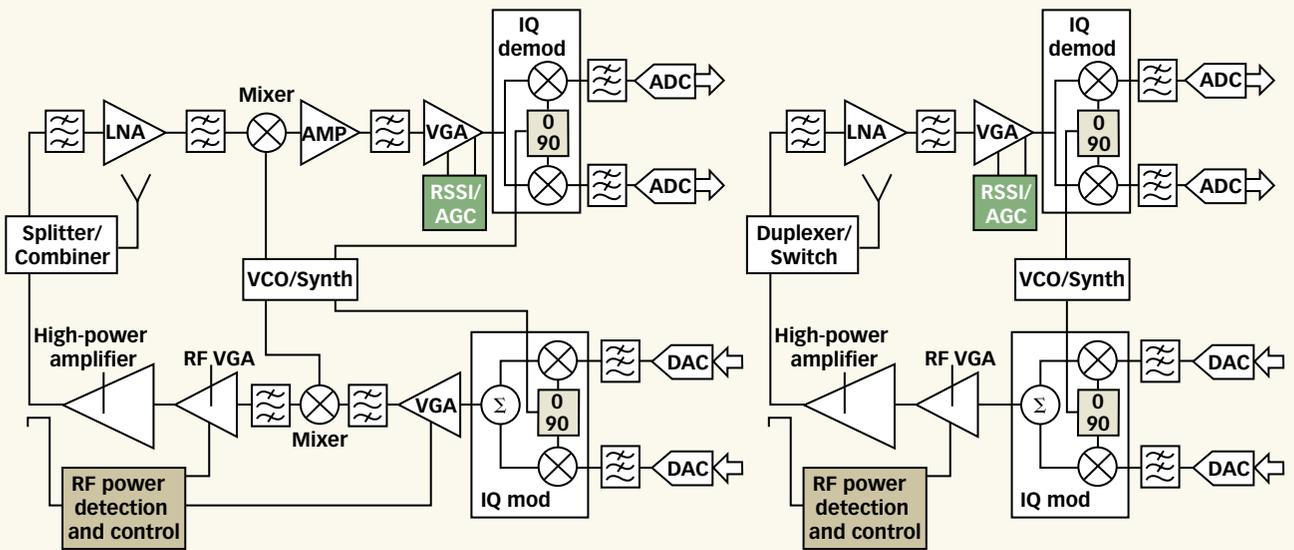
**1. A conventional single-conversion superheterodyne Rx translates the frequency of desired signals through one or more IFs before converting it to baseband. A direct-conversion Rx makes the transition directly from RF to baseband.**
