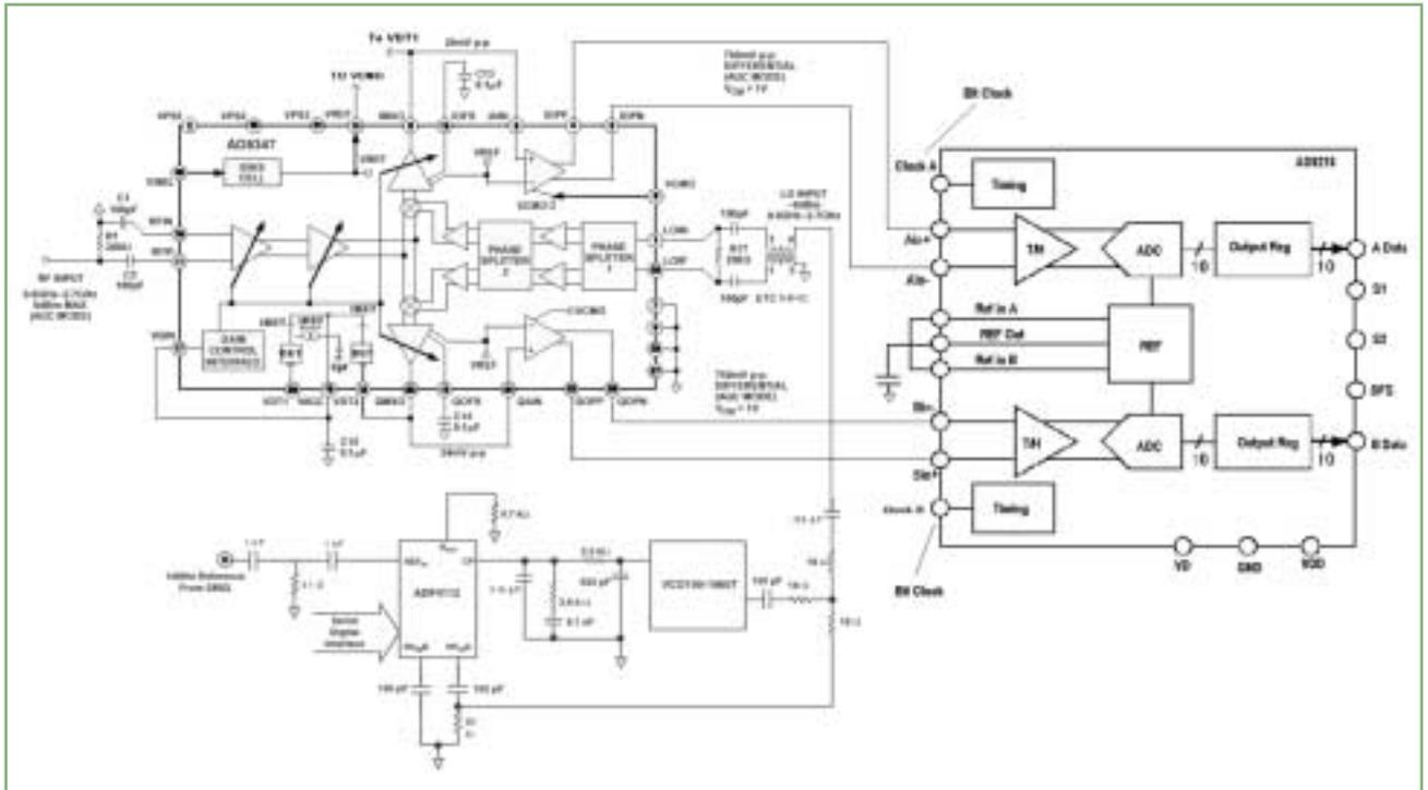
**5. A complete direct-conversion Rx can be assembled using the ADF4112, AD8347, and AD9218 ICs.**
