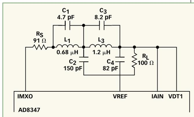
**4. The demodulated output (baseband-mixer output) can be filtered off-chip before being applied to the final baseband amplifiers. The on-chip reference voltage signal (VREF) provides biasing for the filter circuit.**
