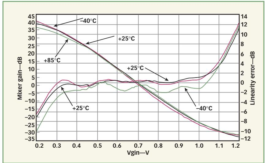
**3. The three-stage VGA (two stages at RF, one stage at baseband) varies gain from  $-30$  to  $+40$  dB. The gain-control function is linear-in-dB over its range.**
