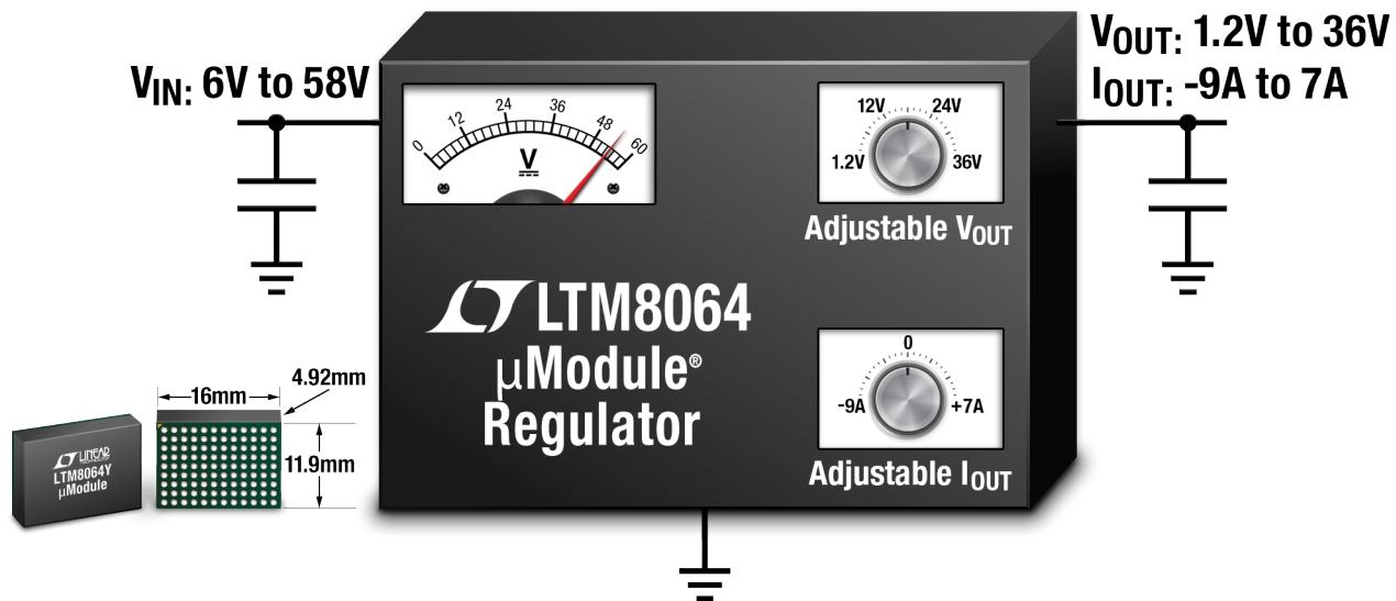
Our constant-voltage, constant-current (CVCC) µModule® regulators provide accurate input current limit in applications such as Peltier devices for cooling and heating, battery and supercapacitor chargers, LED and laser drivers, and motor and fan controllers. These products include a DC/DC controller, MOSFETs, inductor and supporting components in an LGA or BGA package. Only a few resistors, the bulk input and output capacitors are required to complete the design.
