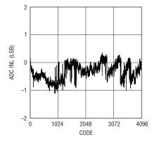
Figure 2. Typical INL error of ADIN voltage is within ±0.5LSB.
