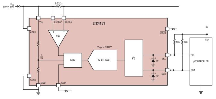
Figure 1. Full featured current and voltage monitor simplifies high voltage, high side sensing.
