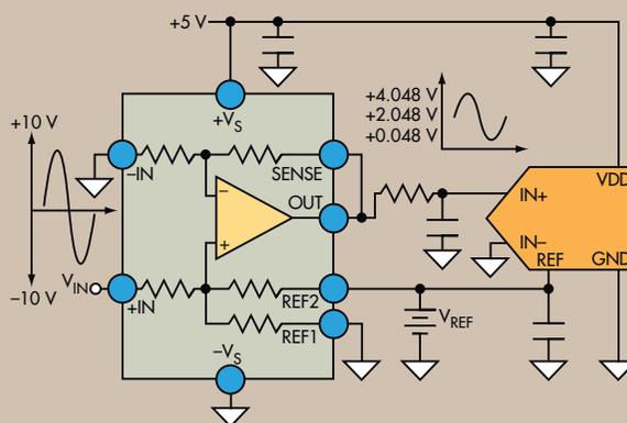
2. A level-translating driver, optimized for specific ADCs, provides a convenient way to accurately match the wide voltage output of sensors excited by  $\pm 10\text{ V}$  (common in industrial applications) to a single-ended ADC input with a more restricted voltage range.
