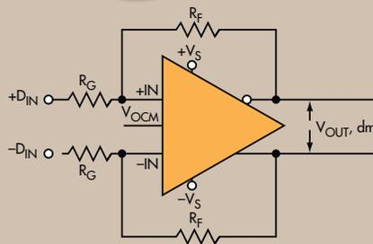
1. Some differential voltage feedback amplifiers include an additional  $V_{OCM}$  input that allows the common-mode voltage of the output signal to be shifted.
