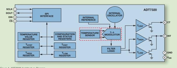
Figure 1. ADT7320 Architecture Diagram
