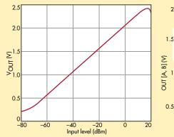
**1**. In a typical output curve for a logarithmic RF power detector, the output is linear over the logarithmic decibel input range.
