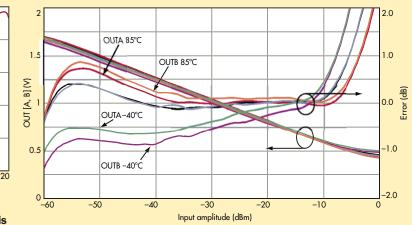
2. This output voltage and temperature error curve of a dual logarithmic RF power detector includes variations from -40°C to 85°C at 2.2 GHz.
