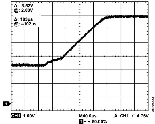
Figure 14. Typical Soft Start Ramp
