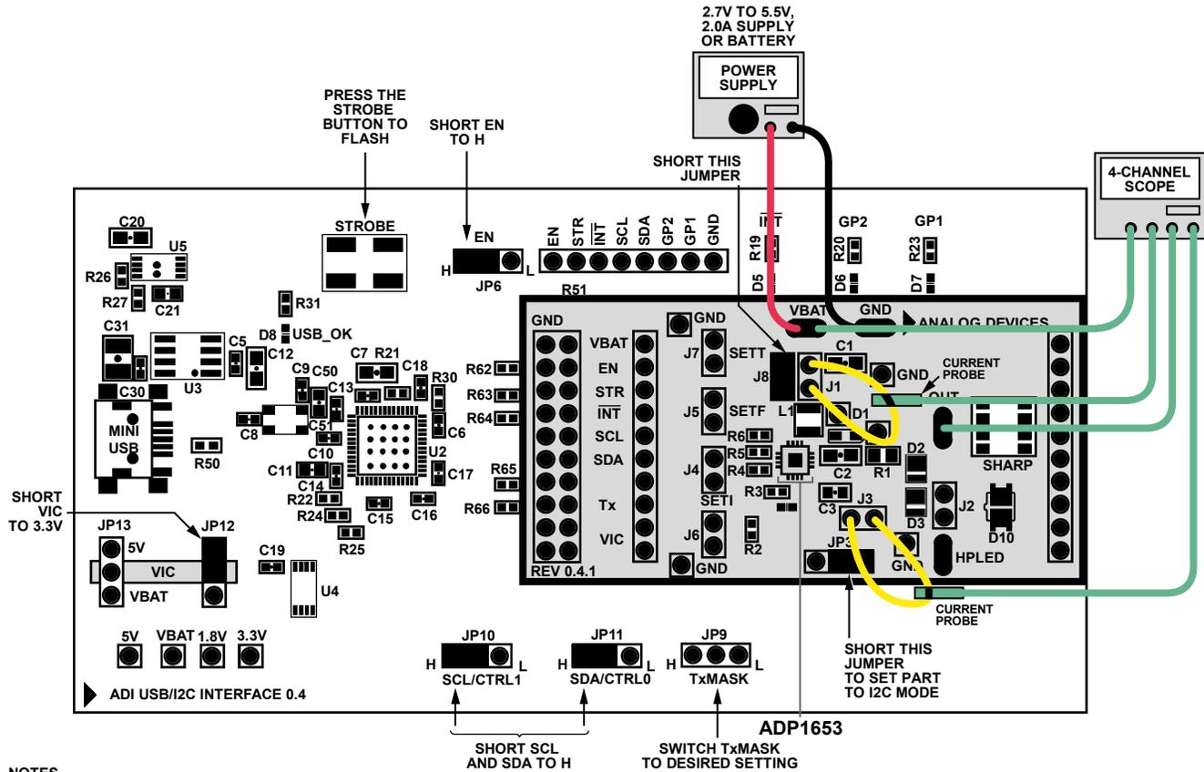
Figure 19. Measuring Current Limit
