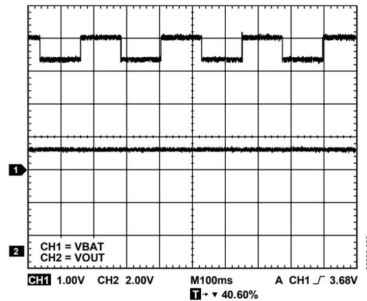
Figure 23. Typical Line Regulation Plot
