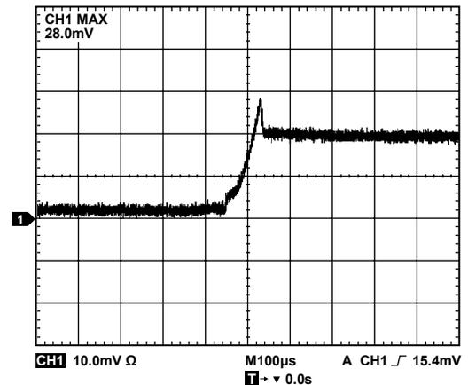
Figure 16. Typical Supply Inrush Current Waveform
