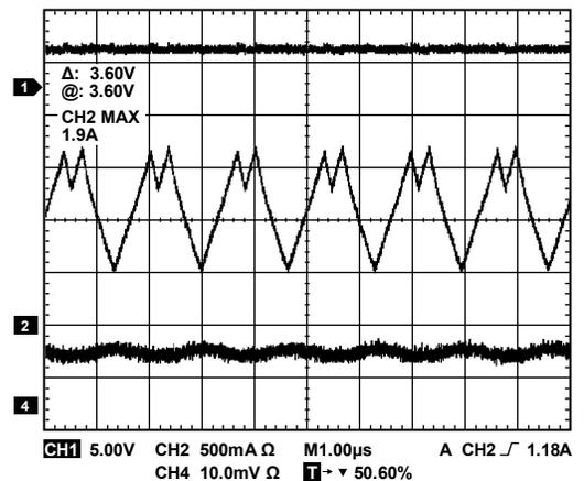
Figure 21. Inductor Current Waveform at Current Limit
