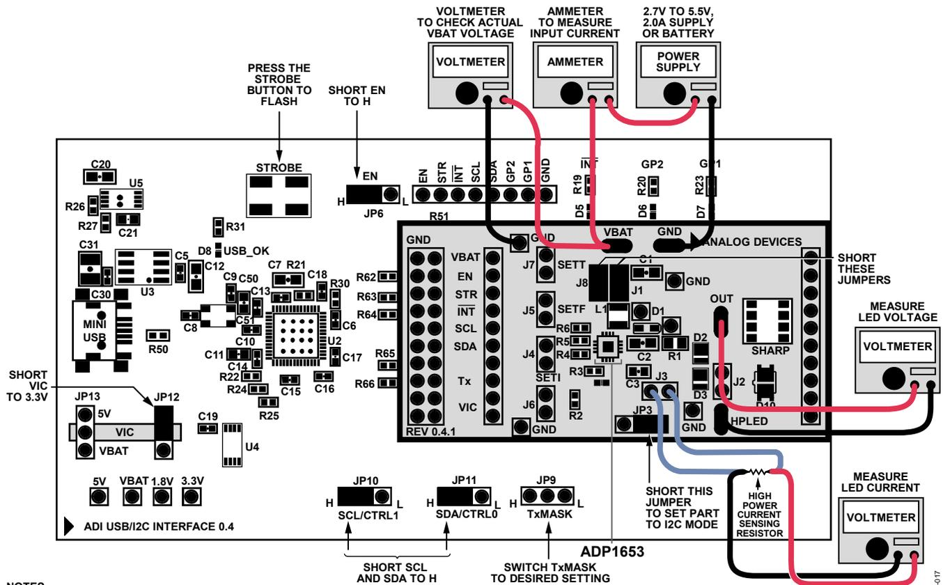
Figure 17. Measuring Efficiency in Torch Mode
