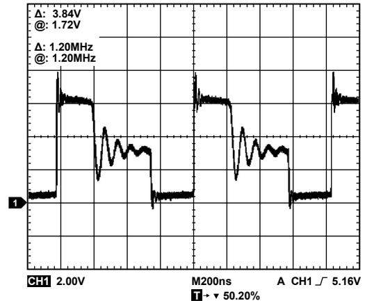
Figure 12. LX Pin, Discontinuous Conduction Mode
