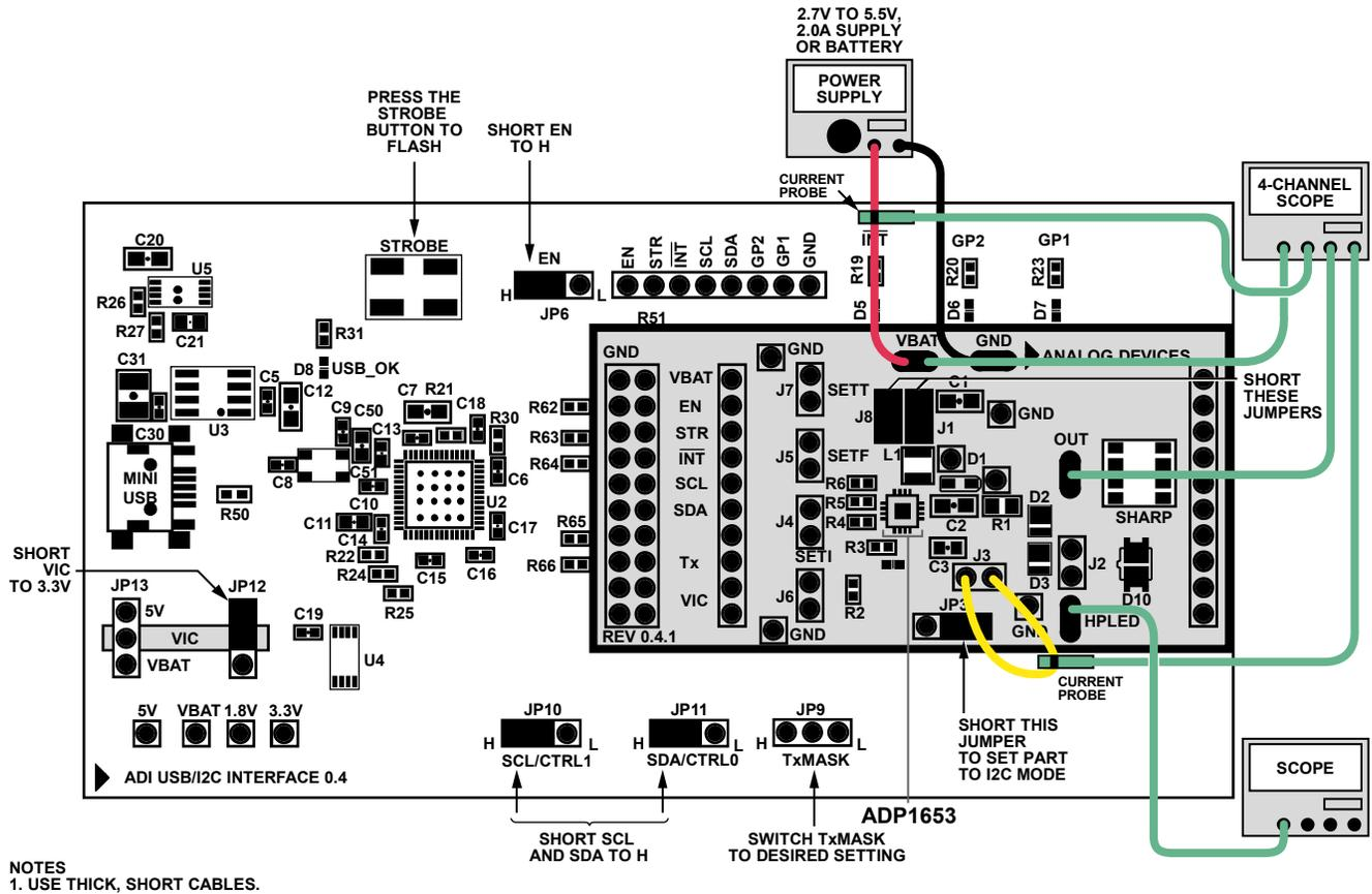
Figure 18. Measuring Efficiency in Flash Mode
