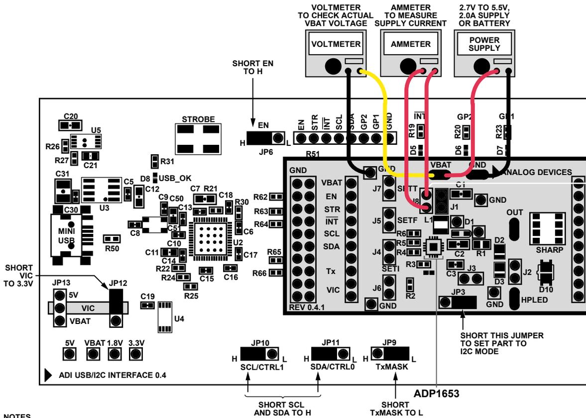
Figure 6. Measuring Supply Current (ILED)
