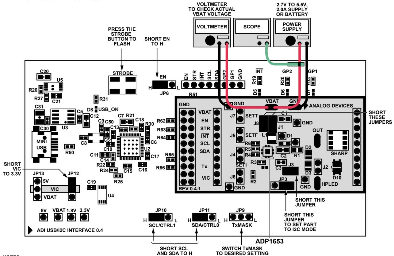
Figure 15. Measuring Inrush Current at Startup
