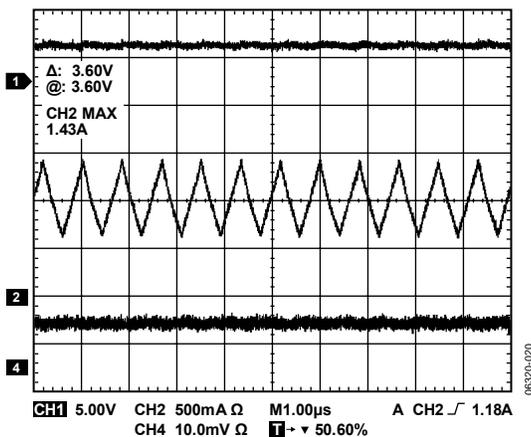
Figure 20. Inductor Current Waveform
