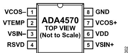
Figure 2. Pin Configuration
