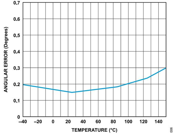
Figure 6. Single Point Calibration Angular Error vs. Temperature
