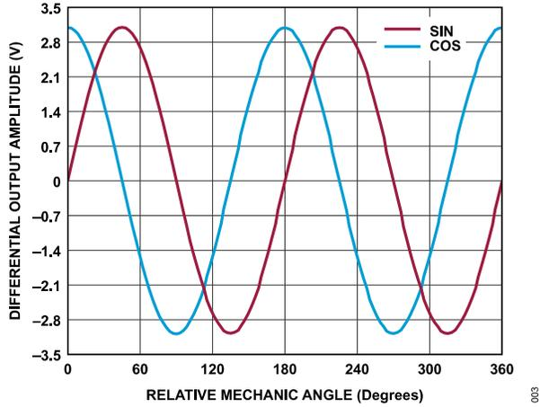
Figure 3. Differential Output Amplitude vs. Relative Mechanical Angle
