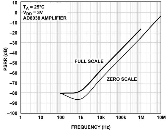
Figure 27. Power Supply Rejection Ratio vs. Frequency
