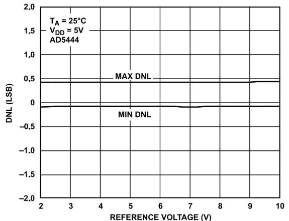
Figure 11. DNL vs. Reference Voltage
