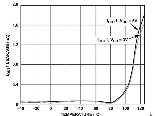
Figure 17. I<sub>OUT1</sub> Leakage Current vs. Temperature
