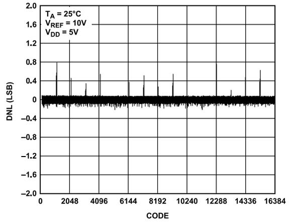
Figure 9. DNL vs. Code (14-Bit DAC)
