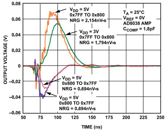
Figure 25. Midscale Transition,  $V_{REF} = 0\text{ V}$
