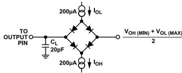
Figure 4. Load Circuit for SDO Timing Specifications
