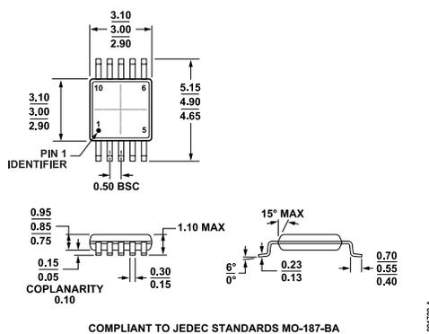
**Figure 53. 10-Lead Mini Small Outline Package [MSOP]
