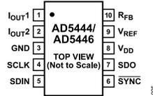
Figure 5. Pin Configuration
