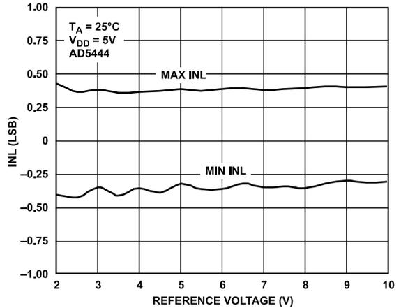
Figure 10. INL vs. Reference Voltage
