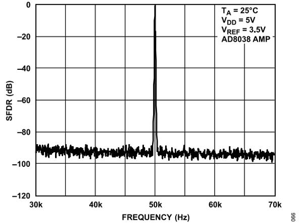
Figure 33. Narrow-Band SFDR,  $f_{OUT} = 50$  kHz, Clock = 1 MHz
