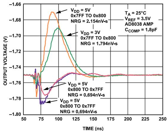
Figure 26. Midscale Transition,  $V_{REF} = 3.5\text{ V}$
