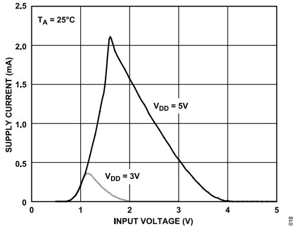
Figure 18. Supply Current vs. Logic Input Voltage
