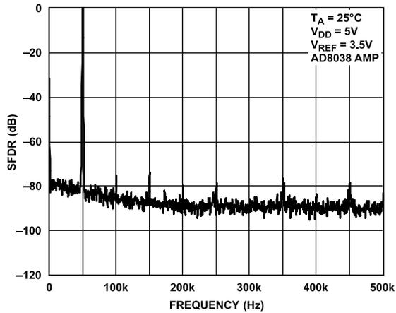
Figure 31. Wideband SFDR,  $f_{OUT} = 50$  kHz, Clock = 1 MHz
