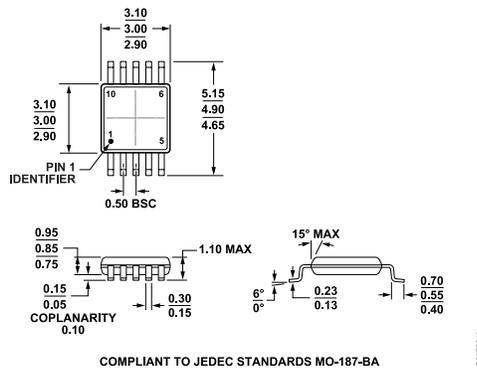
Figure 53. 10-Lead Mini Small Outline Package [MSOP] (RM-10)
