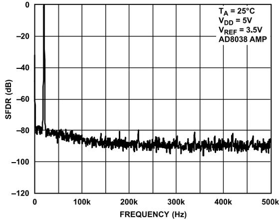
Figure 30. Wideband SFDR,  $f_{OUT} = 20$  kHz, Clock = 1 MHz
