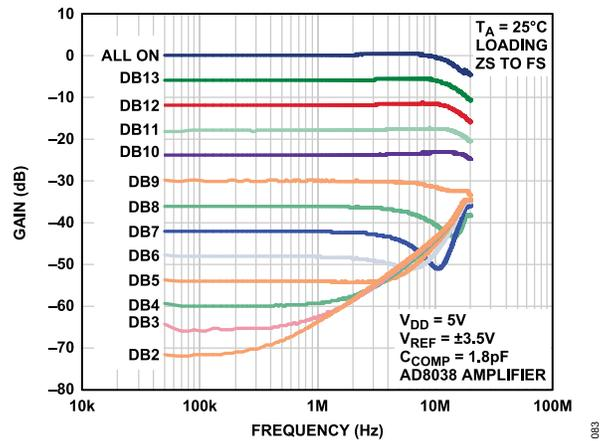
Figure 22. Reference Multiplying Bandwidth vs. Frequency and Code
