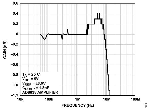
Figure 23. Reference Multiplying Bandwidth vs. Frequency—All 1s Loaded
