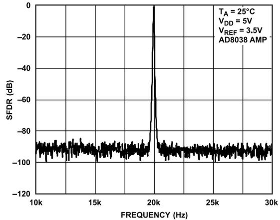
Figure 32. Narrow-Band SFDR,  $f_{OUT} = 20$  kHz, Clock = 1 MHz
