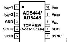
Figure 5. Pin Configuration
