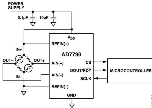
Figure 6. Typical Application Diagram
