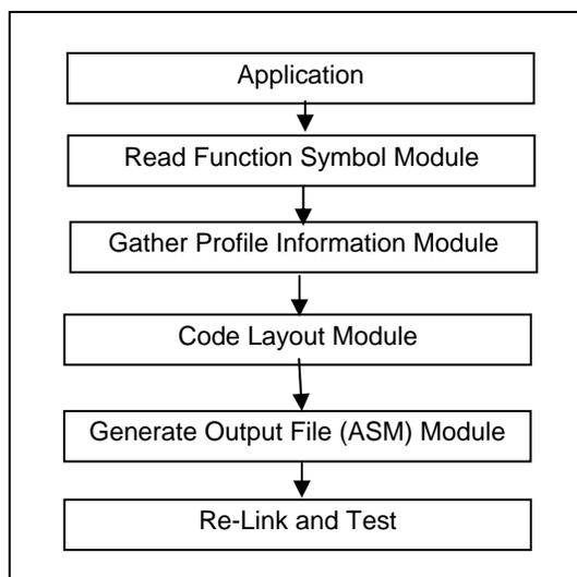
Figure 2. Functional Flow of PGO Linker
