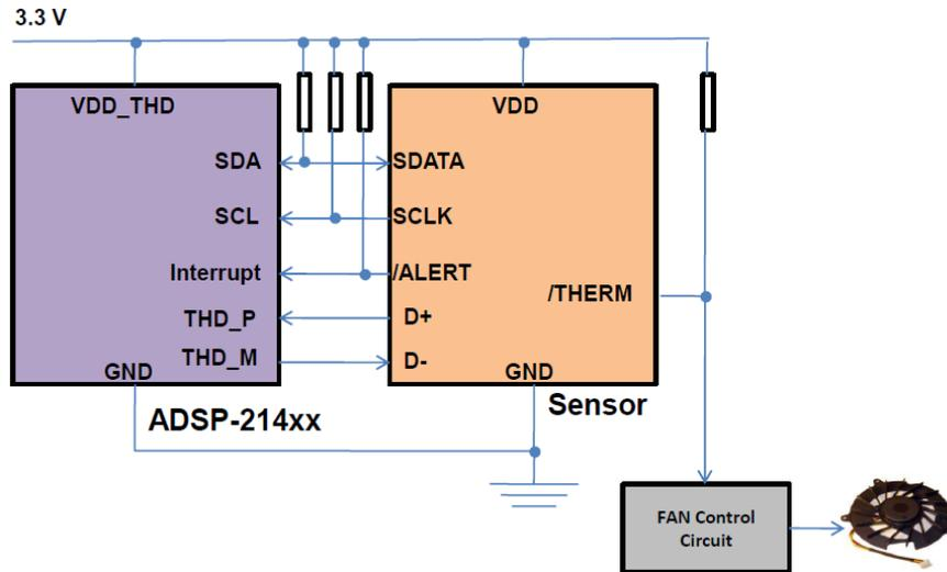
Figure 2. Digital temperature sensor interfaced with an ADSP-214xx processor without a host controller
