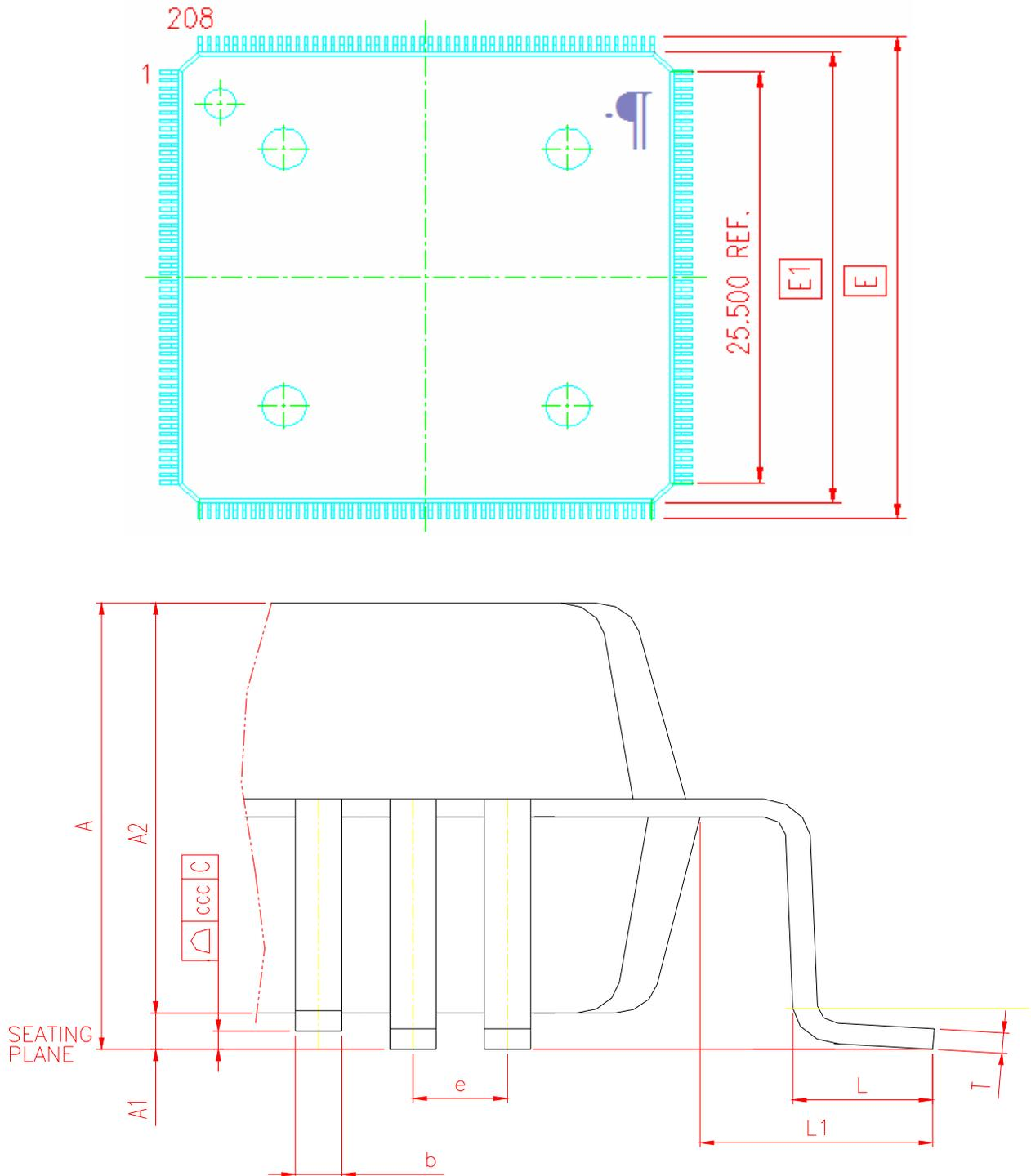
Figure 1. Dimensions of MQFP and LQFP\_EP packages
