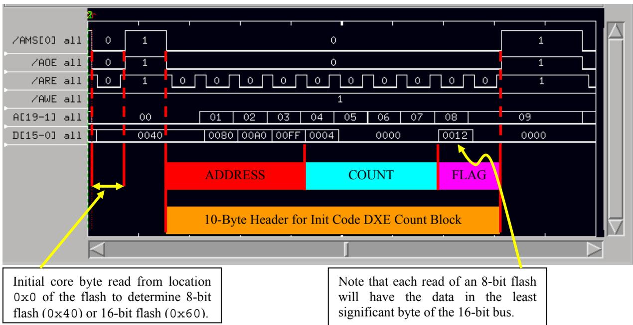
Figure 9. Timing Diagram for 8-Bit Flash Boot Sequence
