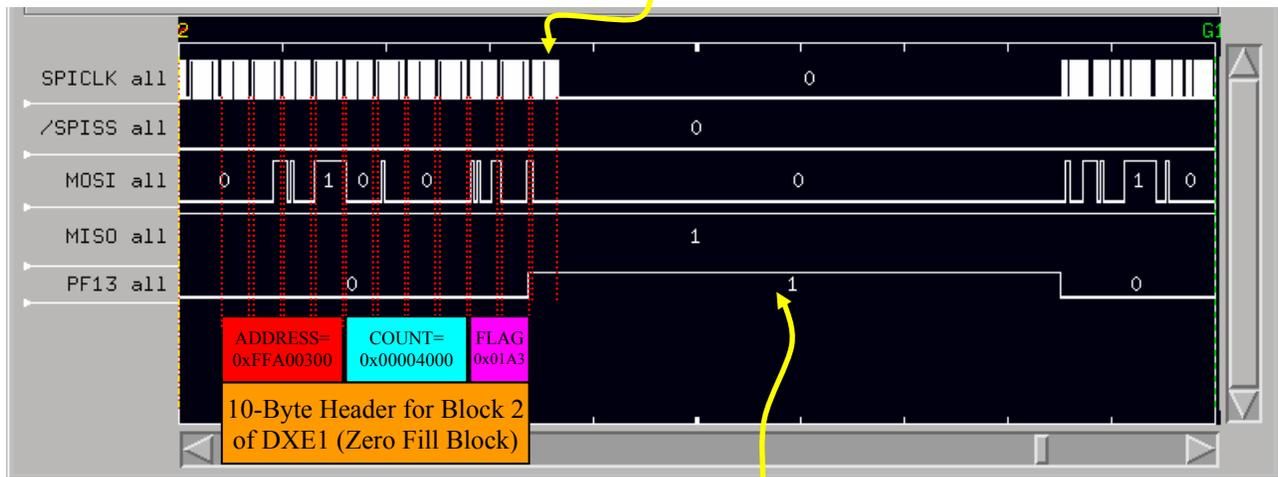
Assertion of HWAIT (PF13) during zero-fill block processing. Processor is zero-filling memory via MemDMA during this time.
