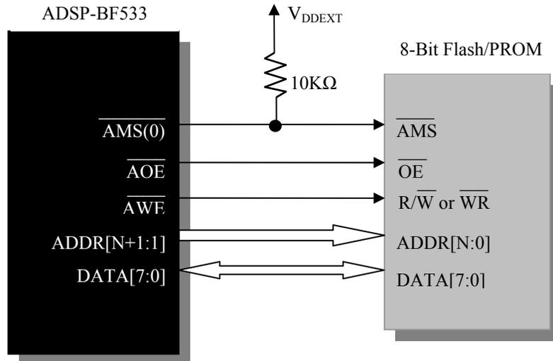
Figure 7. Connections Between a Blackfin Processor and an 8-Bit Flash/PROM
