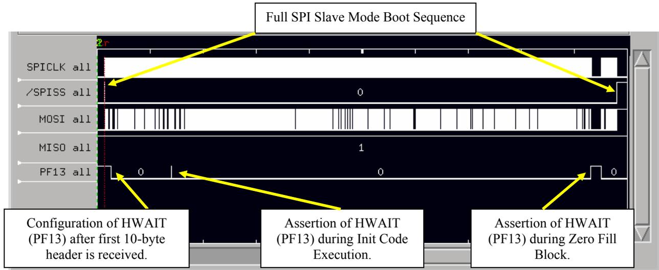
Figure 14. Timing Diagram for SPI Slave Mode Boot Sequence
