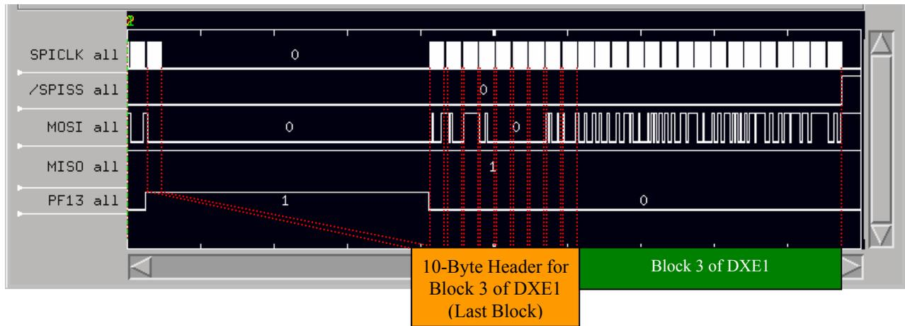
Figure 19. SPI Slave Mode Boot Sequence: Boot Block 3 of DXE1 (Last Block)
