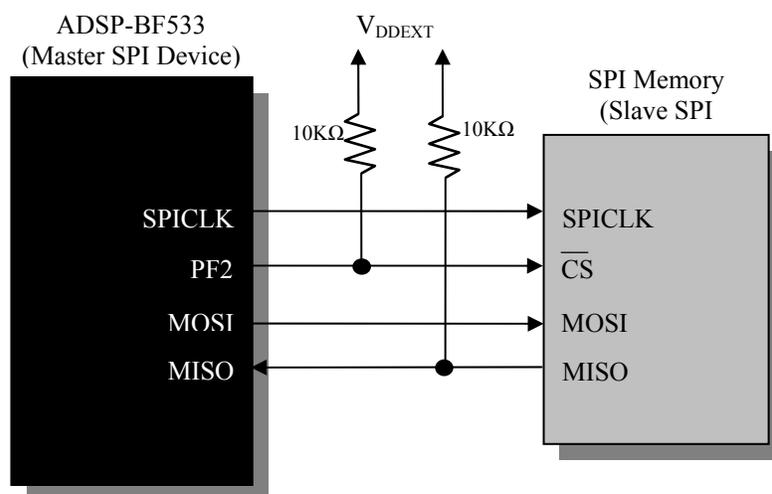
Figure 20. Blackfin – SPI Memory Pin-to-Pin Connections
