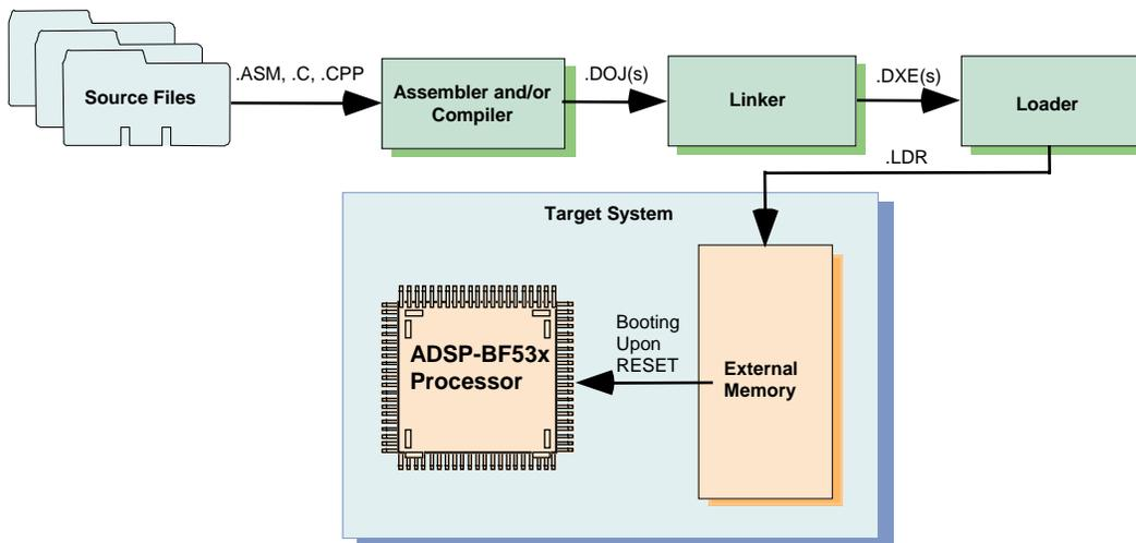
Figure 1. ADSP-BF531/BF532/BF533 Stand-Alone System
