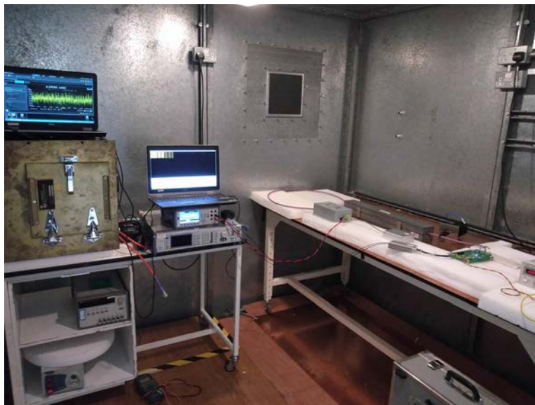
Figure 10. IEC 61000-4-6 Test Setup Photograph
