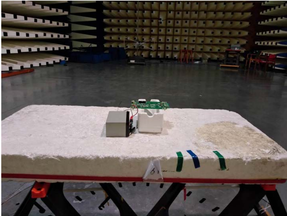
Figure 55. CISPR 11 Test Setup Photograph
