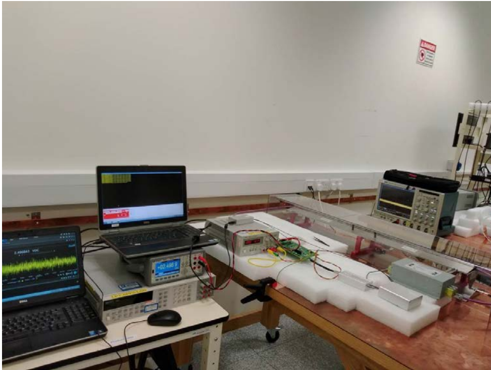
Figure 34. IEC 61000-4 Test Setup Photograph
