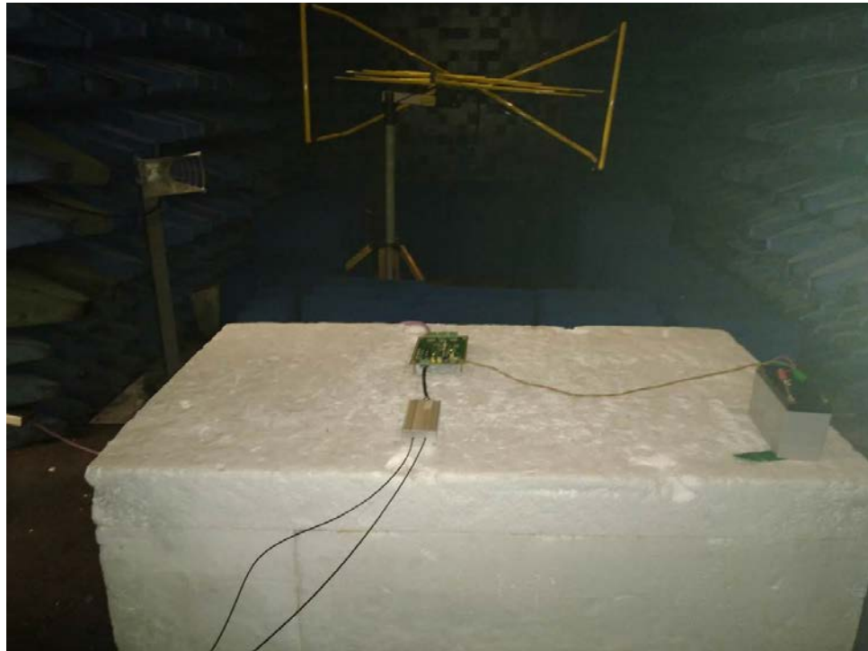
Figure 51. IEC 61000-4-3 Test Setup Photograph
