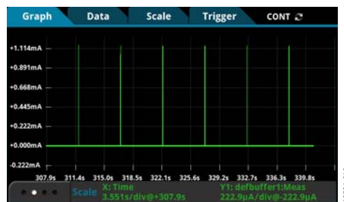
Figure 10. Input Sampling Current Profile Working with the Low Power Water Metering Application
