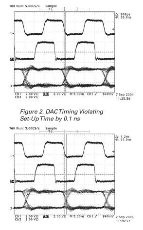
*Figure 3. DAC Timing Violating Set-Up Time by 0.5 ns*
