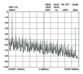
Figure 8. DAC Timing Violating Set-Up and Hold Requirements by 0.5 ns
