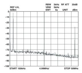
Figure 7. DAC Timing Violating Set-Up and Hold Requirements by 0.1 ns
