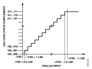
Figure 2. ADC Ideal Transfer Function
