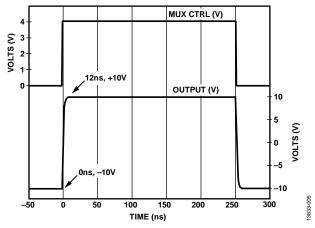
Figure 6. Settling Time Waveforms for the ADG1207 Simulation Model
