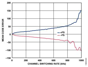
Figure 24. Mean Code Error vs. Channel Switching Rate for Full-Scale Input Step, Gain = 3.2
