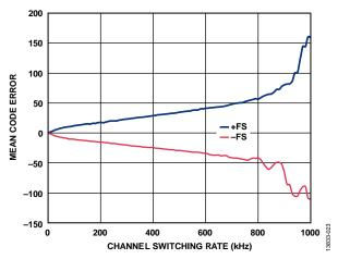
Figure 23. Mean Code Error vs. Channel Switching Rate for Full-Scale Input Step, Gain = 1.6
