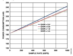
Figure 26. Total System Power Consumption vs. System Sample Rate
