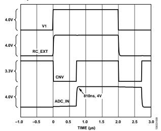
Figure 9. Settling Time Waveforms for the AD7982 and RC Noise Filter
