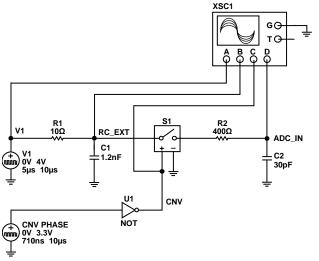
Figure 8. Multisim™ Settling Time Model of the AD7982 and RC Noise Filter
