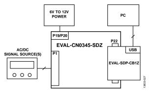
Figure 27. Test Setup Functional Block Diagram
