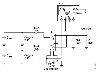
Figure 5. Multisim™ Settling Time Model of the ADG1207
