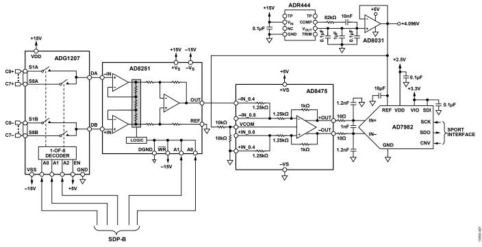
Figure 1. Multichannel Data Acquisition Simplified Circuit (All Connections and Decoupling Not Shown)
