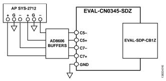
Figure 16. Settling Time Evaluation Setup using AC Signal Generator
