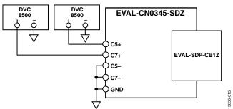
Figure 15. Settling Time Evaluation Setup using DC Calibrators
