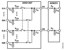
Figure 4. Settling Time Model of the ADG1207
