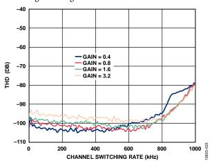
Figure 25. THD vs. ADG1207 Channel Switching Rate for Full-Scale 1 kHz Input
