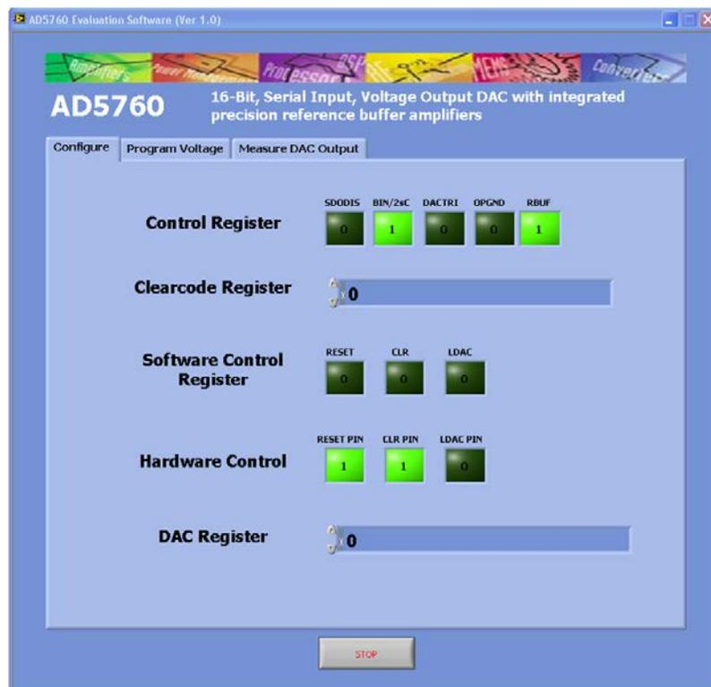
Figure 6. Evaluation Software Main Window
