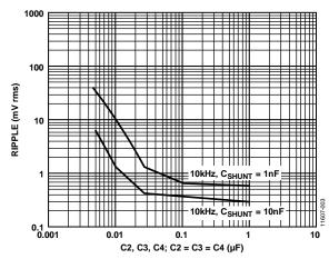
Figure 3. Output Voltage Ripple vs. Filter Capacitance
