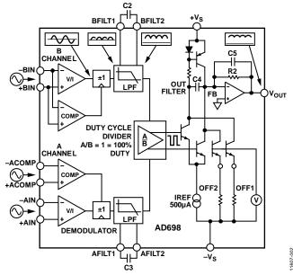
Figure 2. AD698 Block Diagram
