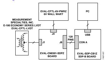
Figure 7. Test Setup Block Diagram
