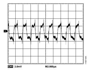
Figure 5. Output Voltage Ripple Before Low-Pass Filter
