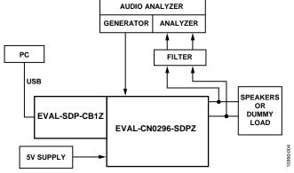
Figure 4. Sound Bar Test SetupDevice Configuration
