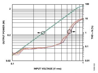
Figure 2. Output Power and THD+N vs. Input Voltage
