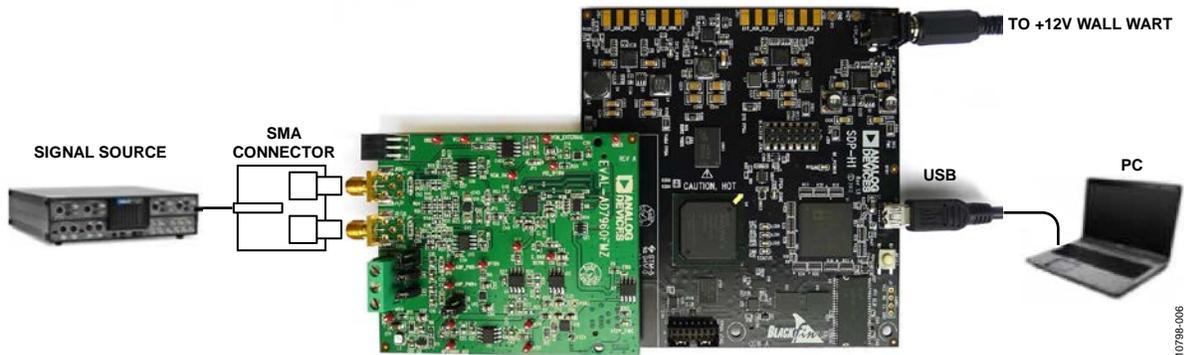
Figure 6. EVAL-AD7960FMCZ Board Connected to EVAL-SDP-CH1Z Board
