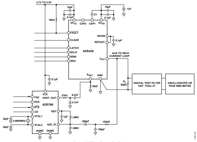
Figure 6. HART Specifications Test Circuit
