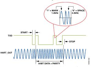
Figure 2. AD5700/AD5700-1 Sample Modulator Waveform
