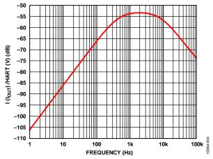
Figure 4. Simulated Frequency Response
