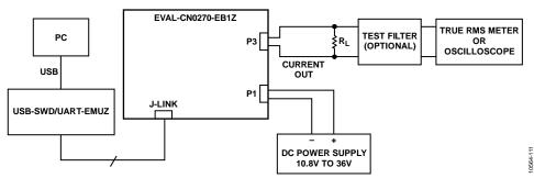
Figure 11. Test Setup Block Diagram
