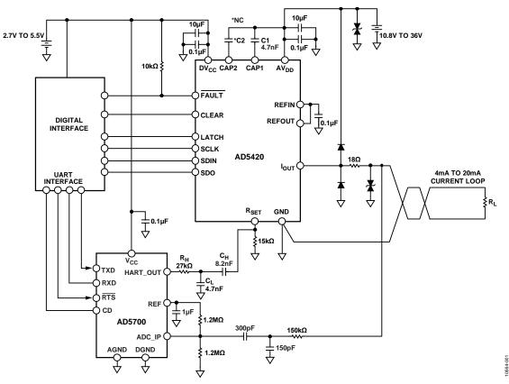
Figure 1. AD5420 HART-Enabled Circuit Simplified Schematic
