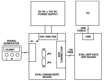
Figure 24. Test Setup Block Diagram
