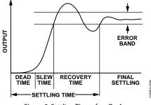
Figure 9. Settling Time of an Op Amp
