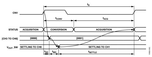
Figure 2. Multichannel Data Acquisition Circuit Timing
