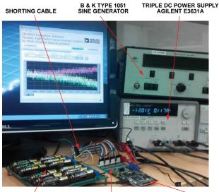
1.5V BATTERY STACK EVAL-CN0269-SDPZ EVAL-SDP-CB1Z Figure 18. Switching Speed and Settling Time Lab Test Setup
