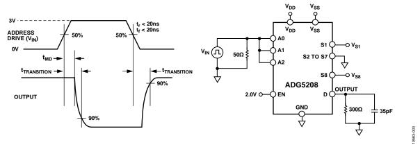
Figure 3. ADG5208 Transition Delay Test Circuit
