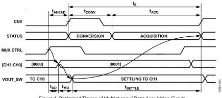
Figure 4. Optimized Timing of Multichannel Data Acquisition Circuit
