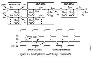
The driver needs to be able to charge the input to the required accuracy (forward-charge) before the switch opens. The backcharge occurs when the switch opens, and generally is short and doesn't present a problem.
