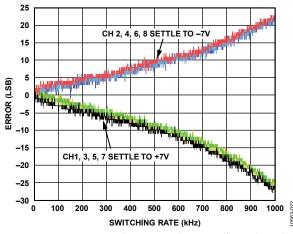
Figure 22. Errors vs. Switching Rate with Front Buffer, 8-Channel Differential Mode, 14 V Step
