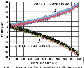
Figure 21. Errors vs. Switching Rate with Input Buffer, 16-Channel Single-Ended Mode, 14 V Step
