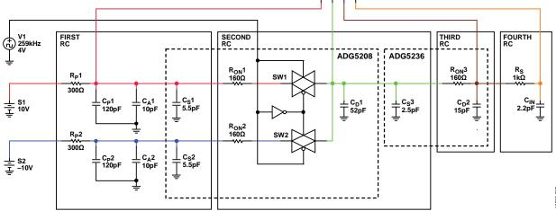
Figure 7. NI Multisim Simulation Circuit for the Pre-Filter, Multiplexer, and AD8065 Input
