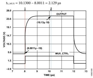
Figure 8. Pre-Filter, Multiplexer, and AD8065 Input Settling Time Simulation
