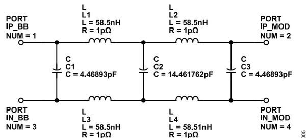
Figure 5. DAC/Mod Interface Filter Topology, 5<sup>th</sup> Order Butterworth, 3 dB BW = 220 MHz, 100 Ω Differential Input and Output Impedance
