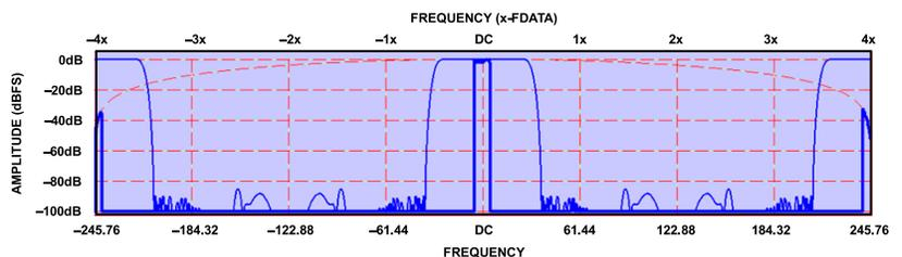
Figure 3. DAC Output Spectrum Using 4× Interpolation, the Thin Blue Line Represents the DAC Interpolation Transfer Function
