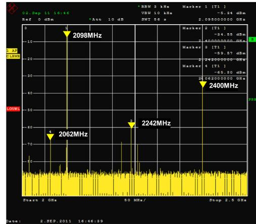
Figure 7. IQ Modulator RF Output with DAC/IQ Mod Filter Absent, LO = 1940 MHz, DAC Input IF = 8 MHz, DAC NCO = 150 MHz, RF = 2098 MHz
