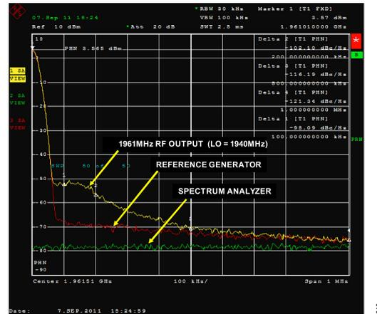
Figure 10. Spectrum Analyzer Noise Floor, Reference Phase Noise, and RF Output Phase Noise
