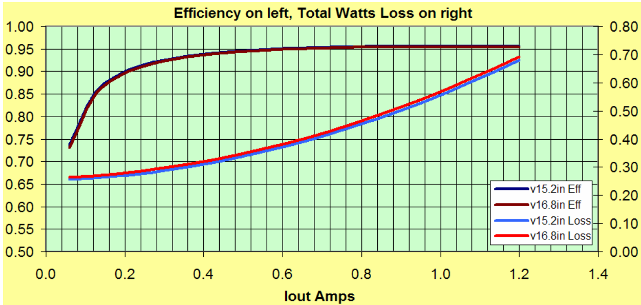
Figure 9. Calculated efficiency of 12.0V output with 1xSi2304BDS high and 1xSi2304BDS low
