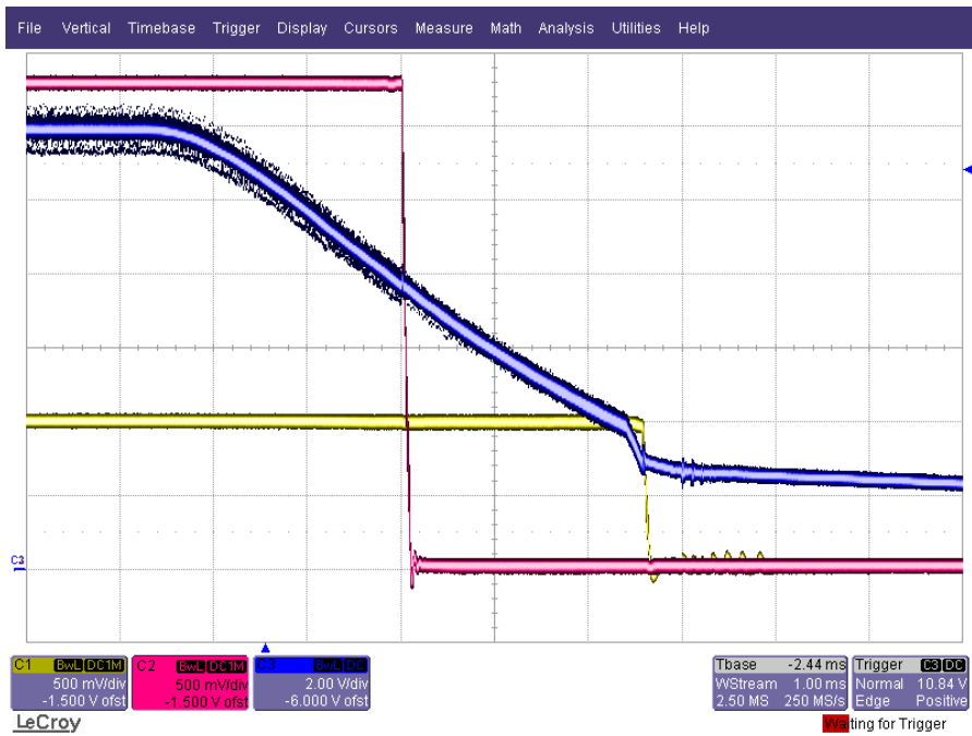
Figure 23. V_{IN} Removed; Ch1 = 1.0 V @ 8 A, Ch2 = 3.3 V @ 1.5 A, Ch3 = V_{IN}
