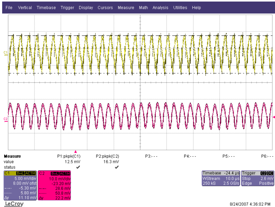
Figure 8. Voltage Ripple V_{IN} @ 10.8 V; Ch1 = 1.0 V @ 0 A, Ch2 = 3.3 V @ 0 A
