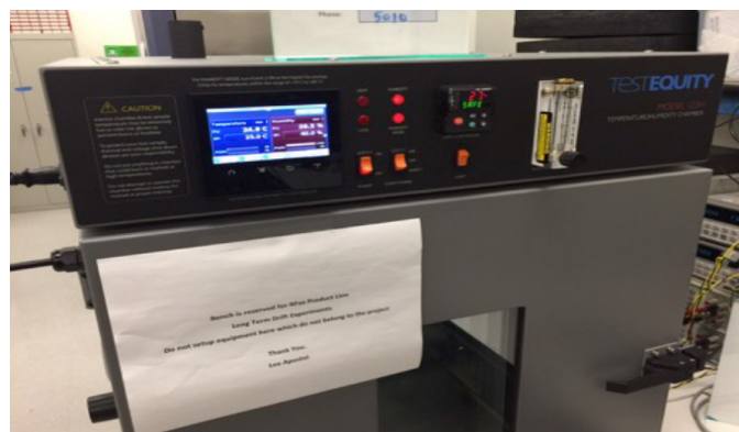
Figure 2. Long-Term Drift Environmental Chamber
